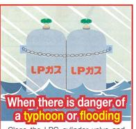
Close the LPG cylinder valve and make sure the cylinder is fastened in place and cannot easily topple over or be washed away.
